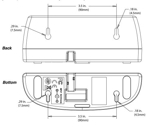
If a metal or wood stud is present, drill a 3/32 inch (2.38mm) pilot hole into the stud and use the supplied #6 x 1 screw to attach the Multi-Bay Charger to the wall. For any of the screws positioned so that they are going directly into dry wall, use a sheet rock anchor/screw set such as the one listed below. Make sure the weight of the power supply is supported separately.
