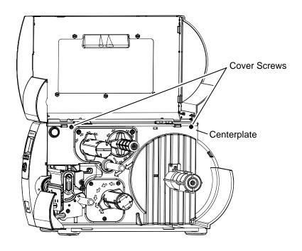
*M*) Tighten the Cover Screws on the Centerplate.
