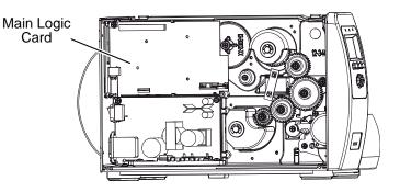
*E*) Remove the Screws that secure the Main Logic Card and the Fill Plate to the Card Cage. Remove the Fill Plate then slide the Main Logic Card out of the printer.
