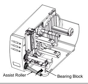
• Insert the Bushing completely into the Bearing Block.
