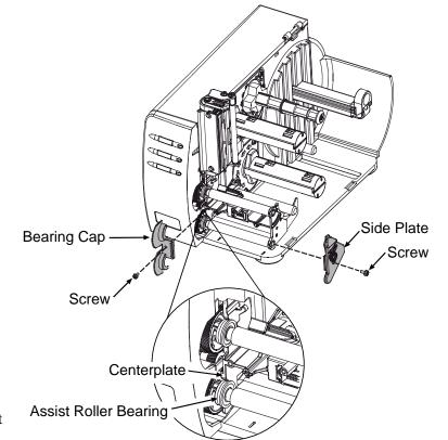
**6** Hold the Bearing Cap in place and secure it with the Screw.
