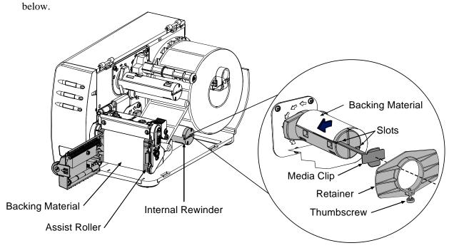
☑ Note: The Media Retainer can be used in place of the Media Clip for a more consistent rewound roll. The Media Clip and Media Retainer cannot be used together.
