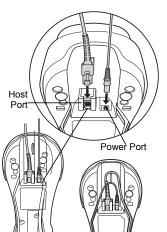
1. Insert the interface cable into the cradle's host port.
