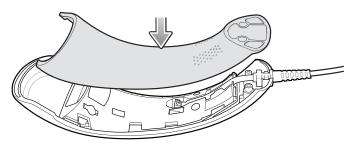
3. Use a Phillips head screw driver No. 1 or 0 to secure the housing of the imager with the two M2.5x11 screws.
