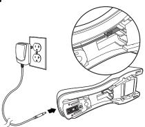
Connect the power adapter to the Charge-Only Base, then plug the power supply into an AC power outlet. Make sure the AC power outlet voltage is the same as the power supply.
