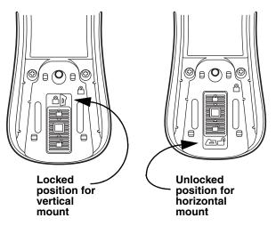
Use 30mm screws, appropriate for the mounting surface material, to mount the base securely.
