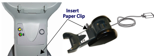
Figure 9. Disconnecting the Cable
