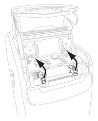
**9.** Remove the platen roller from the printer.
