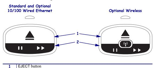
Figure 4 • Control Panel Buttons
