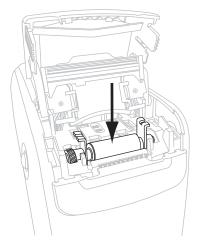
**12.** Secure the platen roller by rotating the two side clips back into place.
