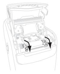
**13.** Align the snap tabs on the bottom of the media chute with the slots in the printer chassis.
