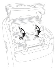
**14.** Press down on the metal lever plate to snap the printhead assembly back into place.
