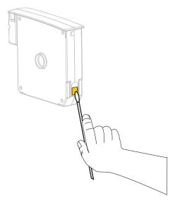
5. Caution • Use only vertical strokes to clean the media cartridge sensor pins. Using horizontal strokes could damage the pins.
