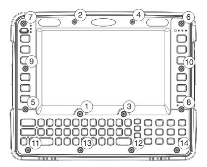
9. Carefully lift the front panel away from the device.
