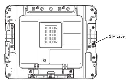
5. Remove the tethered access panel from the opening and press the **UPS battery disconnect** button located just below the SIM card installation slot.
