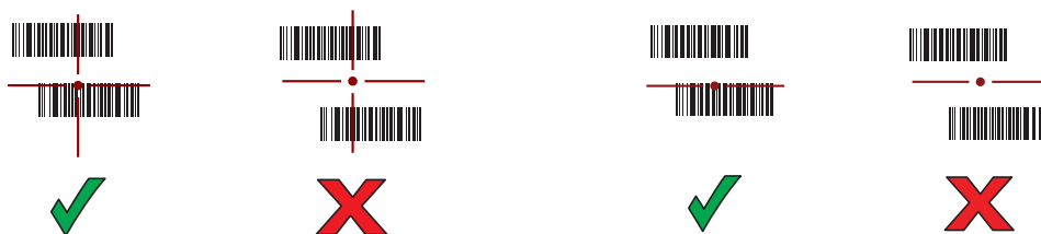
Figure 33 Pick List Mode with Multiple Barcodes in Aiming Pattern: Standard and Extended Range
