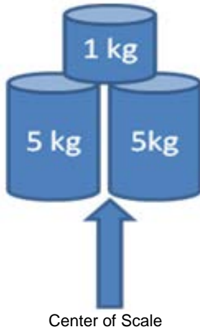
Figure 4-5 Weight Calibration Configuration for Kilograms
