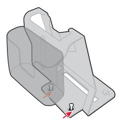
**5** Insert the remaining two screws in the other holes and tighten. Your cart dock is now ready to use.
