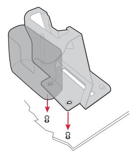
**4** Slide the cart dock to the desired position and then tighten the screws until the cart dock is held firmly in place.
