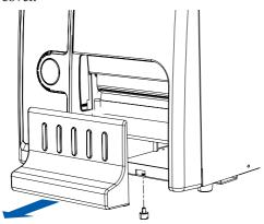
**3** Open the side door and remove the tear bar, held by two Phillips screws.
