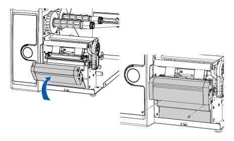
**5** Plug the cutter cable into the connector in the center section as shown. Secure the cable to the bottom plate using the two cable clips included in the kit.
