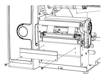
**4** Attach the cutter mechanism to the printer using the two Phillips screws included in the kit.
