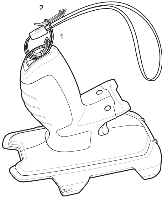
Figure 120 Install Attachment Plate to Handle
