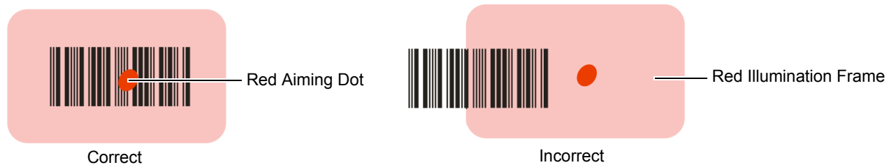
Figure 1-10 Imager Illumination Frame
