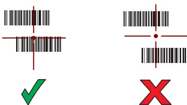
Figure 59: Pick List Mode with Multiple Bar Codes in Aiming Pattern
