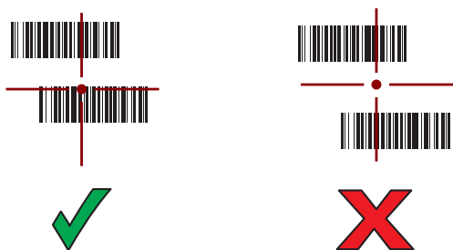
Figure 63: Pick List Mode with Multiple Bar Codes in Aiming Pattern
