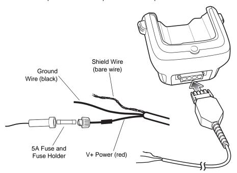
Figure 2-18 Vehicle Cradle Power Connection
