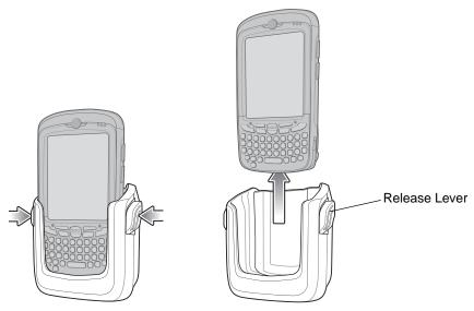
Figure 2-20 Removing the MC55
