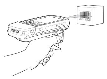
Figure 2-33 Scanning with the Trigger Handle
