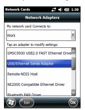
Figure 2-9 Configure Network Adapters Window
