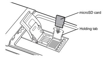
Figure 1-2 Insert microSD Card in Holder
