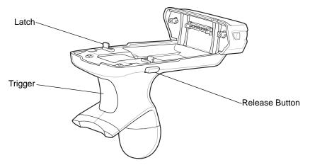
Figure 2-31 Trigger Handle Features
