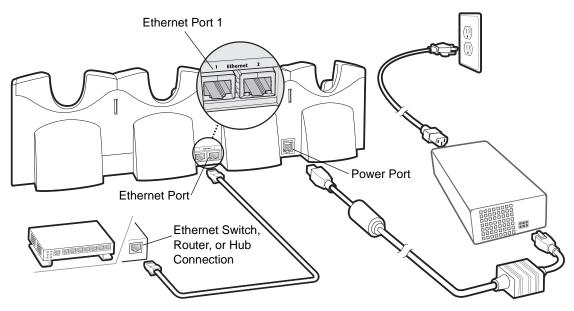
Figure 2-7 Four Slot Ethernet Cradle Connection
