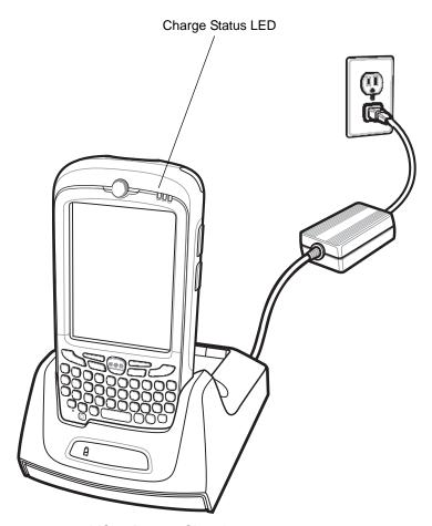
Figure 2-2 MC55 Battery Charging
