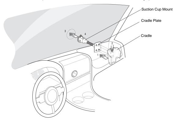
Figure 2-27 Windshield Installation
