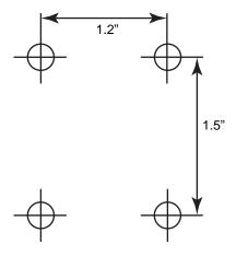
Figure 2-17 Vehicle Cradle Mounting Template
