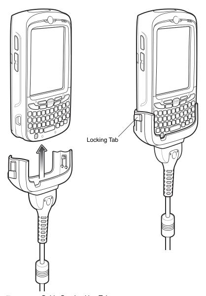
Figure 2-25 Cable Cup Locking Tabs
