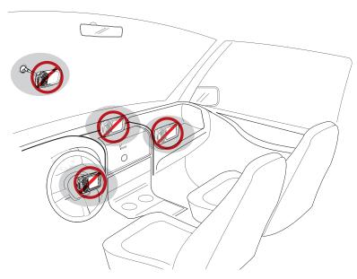
Figure 2-26 Vehicle Holder Mounting
