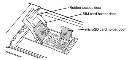
Figure 1-1 Lift SIM Slot Holder Door
