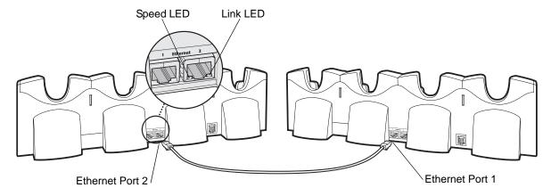
Figure 2-8 Daisychaining Four Slot Ethernet Cradles
