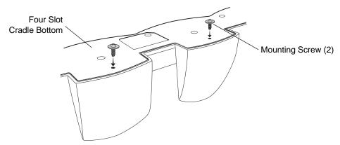
Figure 2-14 Cradle Mounting Screws
