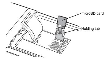
Figure 1-4 Insert microSD Card in Holder
