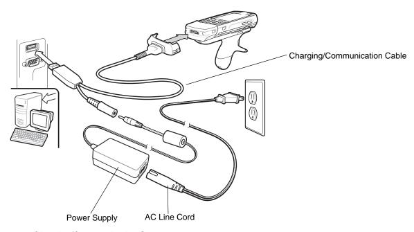
Figure 2-34 Charging/Communication Setup
