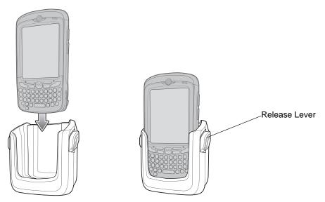
Figure 2-19 MC55 Battery Charging
