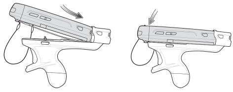
Figure 2-32 Installing the MC55
