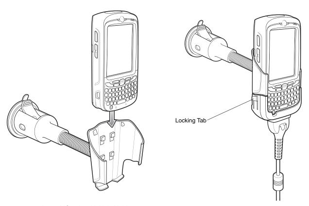
Figure 2-28 Insert MC55 into Vehicle Holder
