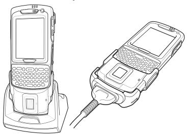
When the reader is placed in a cradle or cable, the reader is inactive and the pass-through is enabled for charging
