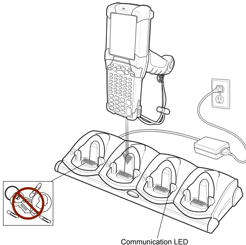
Figure 2-13 Four Slot Ethernet Cradle CRD9101-4001ER
