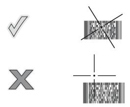
Figure 3-2 Standard Range Imager Aiming Pattern
