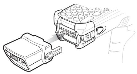
Figure 5-12 Attaching the CAM
