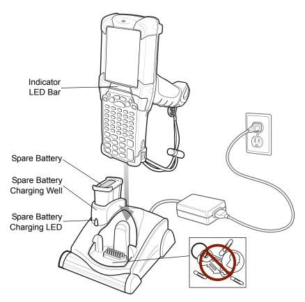
Figure 5-2 Single Slot Serial/USB Cradle
