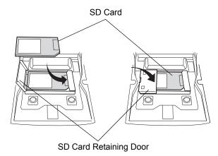
Figure 5-1 Inserting the SD Card
