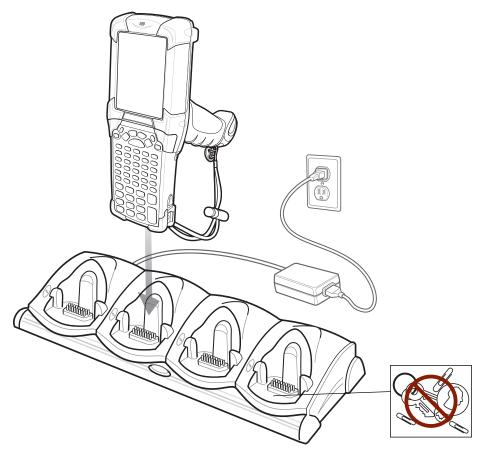
Figure 5-4 Four Slot Charge Only Cradle
