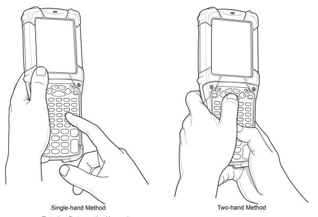
Figure 2-16 Entering Data on the Keypad
