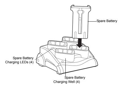
Figure 5-5 Four Slot Spare Battery Charger
