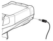
Figure 2-20 Using a Headset (MC9190-G Shown)
