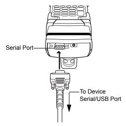
Figure 5-9 MSR Serial/USB Connection
