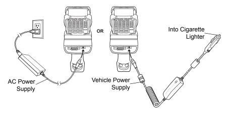
Figure 5-13 CAM Power Connection
