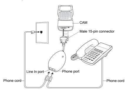
Figure 5-18 Modem Dongle Connection - MC9190-G
