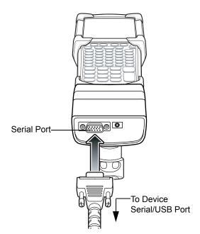
Figure 5-14 CAM Serial Connection
