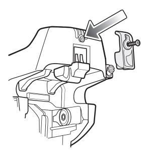
Figure 5-23 Locking Mechanism
