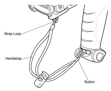
Figure 1-4 Reposition the Strap
