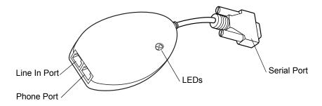
Figure 5-17 Modem Dongle
