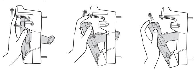
Figure 5-22 Remove MC9190-G from Forklift Cradle
