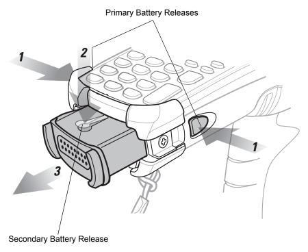
Figure 1-3 Removing the Main Battery
