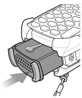
Figure 1-2 Installing the Main Battery
