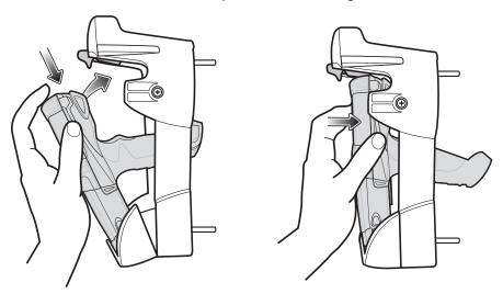
Figure 5-21 Insert MC9190-G into Forklift Cradle
