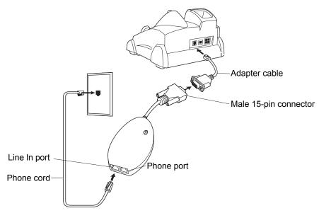
Figure 5-19 Modem Module Connection - Single Slot Serial/USB Cradle
