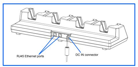
The ST4004 Quad Docking Station is designed to accept up to four Omnii hand-held computers. The docking station powers the units and their internal battery charger. The docking station also connects up to four of the hand-held computers to a 10/100 Base-T Ethernet network and allows for Ethernet data transfer. An additional Ethernet interface is available for connecting more docking stations downstream, up to 4 on the same network.
