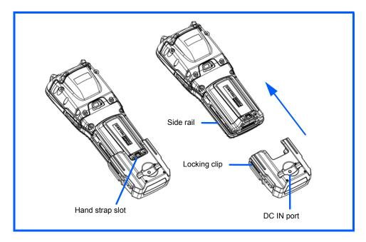
To attach the Snap Module charger to Omnii:
