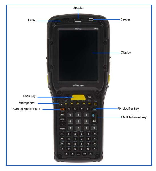
Figure 1-1 Front View of the Omnii XT15 Model with Alphanumeric Keyboard
