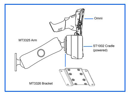
To accommodate the service loop of the connector cable, leave a 4" clearance at the bottom of the cradle. Leave a 7" (minimum) clearance at the top of the cradle to allow easy removal of the hand-held. Refer to the detailed assembly instructions that are packaged with the cradle when selecting a mounting location (*Omnii Vehicle Cradles Quick Start Guide PN 8000221*).
