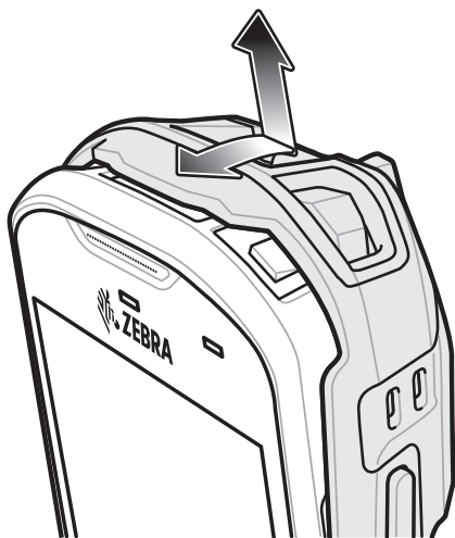
Figure 6-45 Lift Boot Over Device
