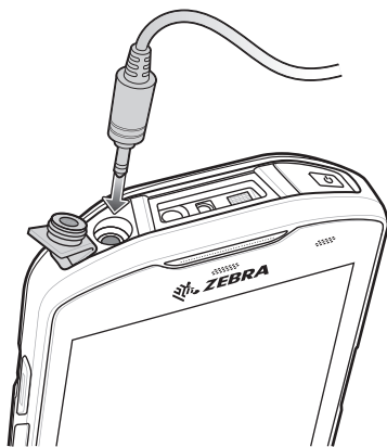
Figure 6-33 Audio Adapter Installation
