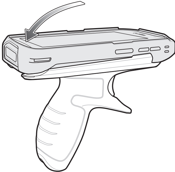
Figure 6-49 Rotate Device onto Trigger Handle
