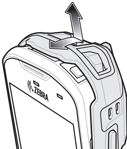
Figure 6-17 Lift Boot Over Device
