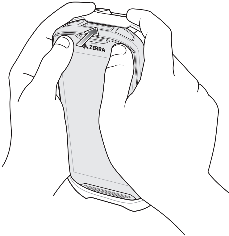
Figure 6-46 Push Device into Boot
