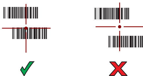
Figure 5-9 RS507 Pick List Mode with Multiple Bar Codes in Aiming Pattern
