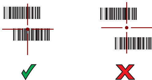
Figure 5-6 Internal Imager Pick List Mode with Multiple Bar Codes in Aiming Pattern
