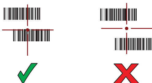
Figure 5-12 RS6000 Pick List Mode with Multiple Bar Codes in Aiming Pattern
