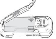
5. Place the hand strap clip into the hand strap attachment slot and pull down to lock into
