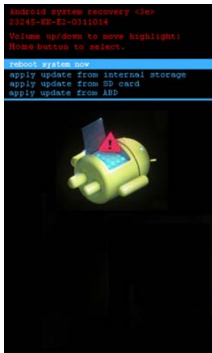
Figure 1-11 System Recovery Screen
