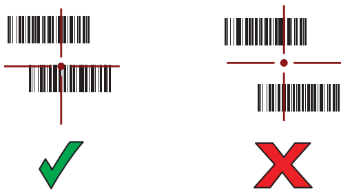
Figure 3-12 Pick List Mode with Multiple Bar Codes in Aiming Pattern
