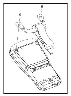
• Stretch the hand strap toward the base of the WORKABOUT PRO<sup>3</sup>, and hook the bottom of the strap into the slot near the base of the battery pack. A tethered stylus and optional external stylus tube can be attached to the hand strap as illustrated below
