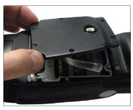
• Fasten the new back plate onto the WORKABOUT PRO<sup>3</sup> using the supplied screws (PN 9009770).
