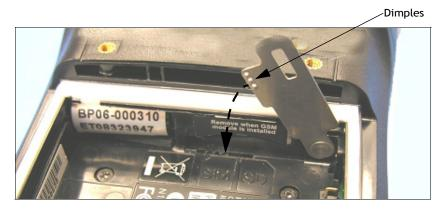
• Push the door down so the dimples fit into the slot cut into the battery compartment plastic.
