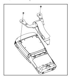
• Stretch the hand strap toward the base of the WORKABOUT PRO<sup>3</sup>, and hook the bottom of the strap into the slot near the base of the battery pack. A tethered stylus and optional external stylus tube can be attached to the hand strap as illustrated below
