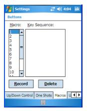
A macro has 20 programmable characters (or "positions"). The macro keys can be programmed to replace frequently used keystrokes, along with the function of executable keys including [ENTER], [BKSP] and [DEL] ([FN/BLUE]-[BKSP]), function keys, and arrow keys.
