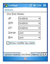
The options in this tab allows you to determine how modifier keys on your WORKABOUT PRO<sup>3</sup> behave. For each modifier key–[ALT], [SHIFT], [CTRL], [FN/ORANGE] and [FN/BLUE] – you have the following options in the drop-down menu: Lock, OneShot, and OneShot/Lock.
