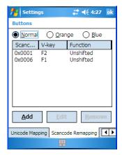
The first column in the *Scancode Remapping* tab displays the Scancodes in hexidecimal. If the scancode is remapped to a virtual key, that virtual key is displayed in the next column labelled 'V-Key'. A virtual key that is 'Shifted' or 'Unshifted' is displayed in the third column labelled 'Function'
