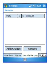
The *Unicode Mapping* tab is used to map combinations of virtual key values and [CTRL] and [SHIFT] states to Unicode<sup>™</sup> values. This tab shows the configured Unicode character along with the Unicode value. For example, "a (U+0061)" indicates that the character "a" is represented by the Unicode value "0061", and so on. Keep in mind that Unicode configurations are represented as hexidecimal rather than decimal values.
