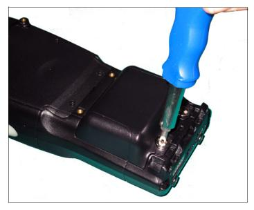
• To *lock* the secure battery cover, fit the spanner into the latch dimples, and turn the spanner until the dimples are aligned horizontally.
