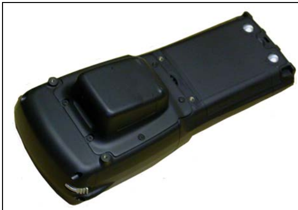
Figure 8.3 The Scanner Pod In Place
