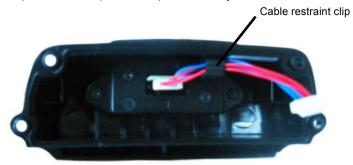
**NOTE** Ensure that the end-cap cables are threaded through the cable restraint clip.
