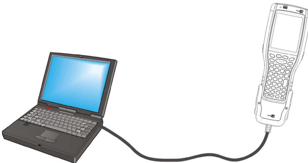
Figure 11: Direct Data Communication Using Snap-on Cable
