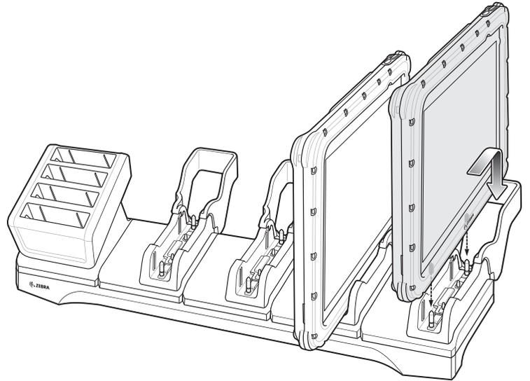
3. Place the ET5X down into the slot with display facing away from Battery Charger.
