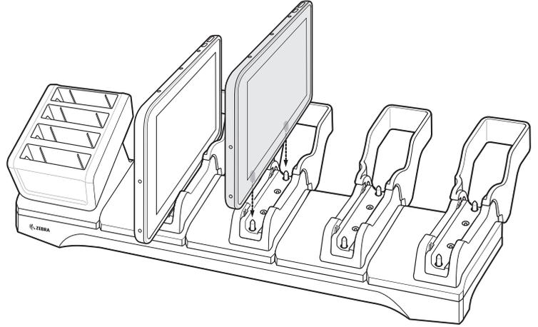
3. Place the ET5X down into the slot with display facing away from Battery Charger.
