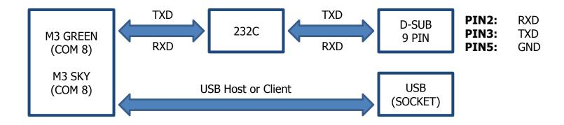
Switch ON:Serial communication and USB Host can be used.Switch OFF:USB Client is possible.
