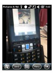
While the camera application is running, click on Capture button or press 'C' button (right-up side key) to capture the image. You should be able to check the result straight after the capture. Captured image is saved in the same folder (default path) as the camera application.
