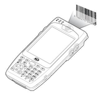
Make sure the laser beam covers whole barcode to read data properly.
