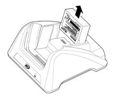
Remove the spare battery from the charging slot when charging is done.
