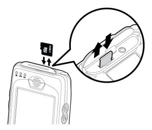
To insert MicroSD, first open the top cover and slide in the external memory card in the right direction until you feel a click.
