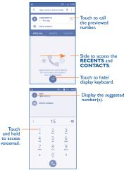
Enter the desired number from the keyboard directly and touch  $\int_{-\infty}^{\infty}$  to place the call or select a contact from **CONTACTS** or **RECENTS** by sliding or touching tabs, then choose your target SIM card to make the call.
