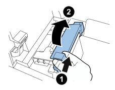
Open Transport Guide and slide it in the arrow direction.
