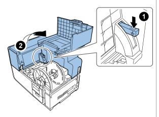
9. Remove shipping tapes and cushioning materials from inside of Printer.
