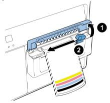
When Optional Cutter Unit is installed, the paper is automatically cut.
