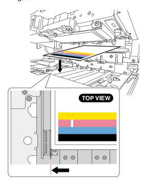
9. Identify the position of non-discharging nozzle(s) depending on the corresponding position of the white streak(s).
