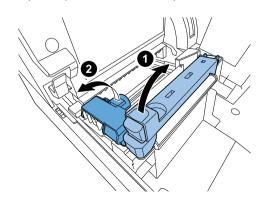
Insert Test Label along the left-side guide under TOF Sensor until it stops at the roller in the feeder slot.
