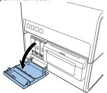
2. Open Ink Tank Lever for each color while pushing it downward.
