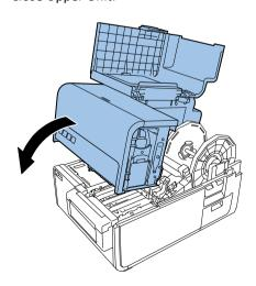
3. Remove the shipping tape, remove Print Module Cover, and then open Lower Printhead Release Lever.
