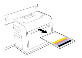
7. Observe printed Nozzle Check Pattern. In the case that white streak is in solid printed area, execute strong cleaning once. Refer to the table 1 in step 4.
