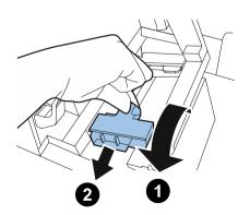
4. While pressing Jam Release Lever down, pull out paper.
