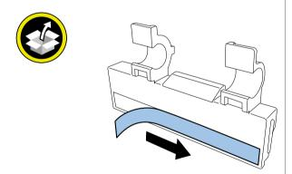
10. **For CPX4P,** attach Scraper to Printhead.
