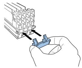
11. Put Printhead Unit on the rail guide, and then insert it into Printer until it stops.
