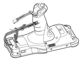
3. Attach the two plastic ends together.
