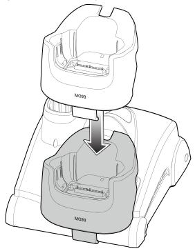
4. Insert the device into the cradle.
