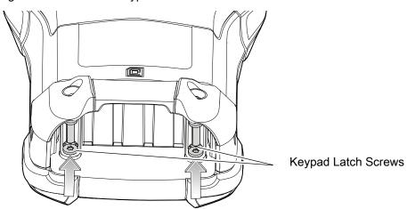
4. Slide the keypad latches toward the bottom of the device.
