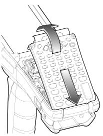
13. Using a Torx T8 screwdriver with a large grip and a long shaft, secure the keypad to the device using the two screws. Torque screws to 5.8 kgf-cm or 5.0 lbf-in.
