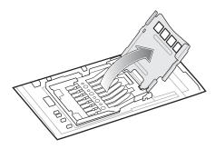
10. Insert the microSD card into the card holder door ensuring that the card slides into the holding tabs on each side of the door.
