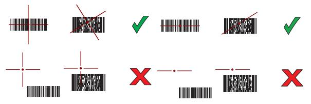
Figure 74 Pick List Mode with Multiple Barcodes in Aiming Pattern: Standard and Extended Range
