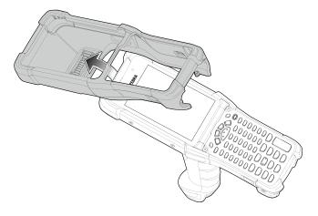
2. Grasp the bottom of the rubber boot and place over the bottom of the device.
