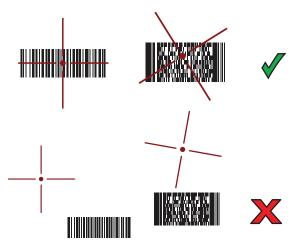
Figure 82 RS6000 Pick List Mode with Multiple Barcodes in Aiming Pattern
