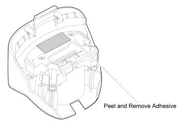
3. Insert the adapter into the MC9XXX cradle and adhere to the bottom of the cradle.
