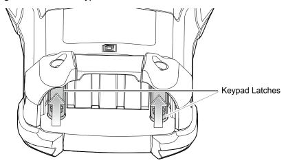
12. Using a Torx T8 screwdriver, replace the two keypad latch screws inside the battery slot and torque to 5.8 kgf-cm or 5.0 lbf-in.
