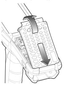
9. Using a Torx T8 screwdriver with a large grip and a long shaft, secure the keypad to the device using the two screws. Torque screws to 5.8 kgf-cm or 5.0 lbf-in.
