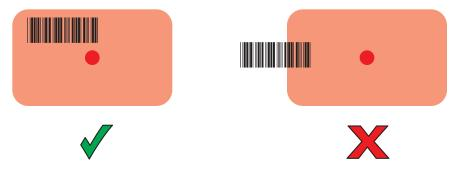
Figure 85 DS3608/DS3678 Pick List Mode with Multiple Barcodes in Aiming Pattern
