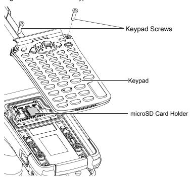
7. Lift the keypad from the device.
