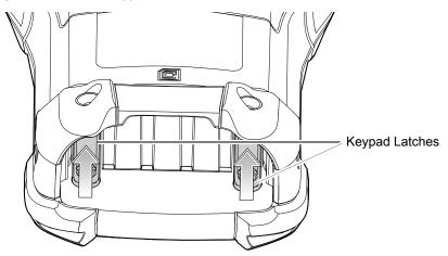
16. Using a Torx T8 screwdriver, replace the two keypad latch screws inside the battery slot and torque to 5.8 kgf-cm or 5.0 lbf-in.
