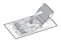
12. Align the keypad along the bottom ridge of the device, and then lay it flat.
