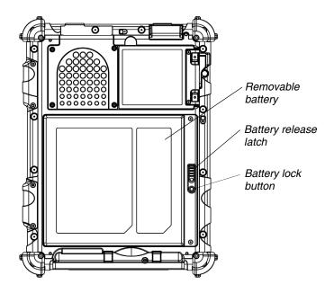
**3.** Pull the battery away from the computer and remove it.
