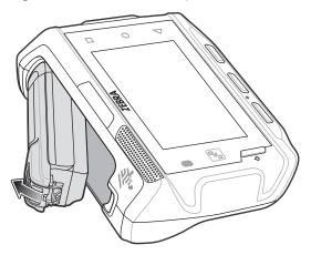
Figure 8 Extended Battery Removal
