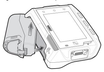
5. Press the battery down until it snaps into place.
