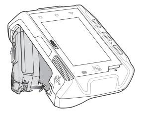
Figure 4 Extended Battery Installation
