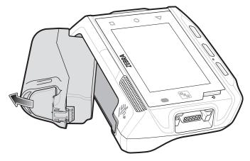
4. Insert the end of the battery into the battery well.
